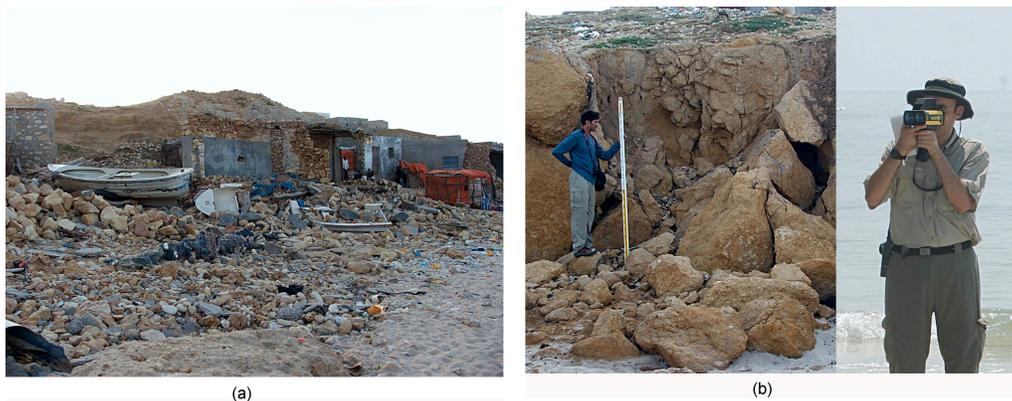
**Figure 7.** Bandarbeyla: (a) boats smashed ashore amidst house rubble; (b) surveying of shore erosion with a laser rangefinder.
